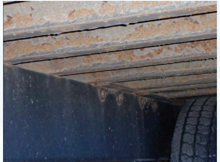
Truck Trailer with Frame Rail Coated, Bed Supports Un-Coated
